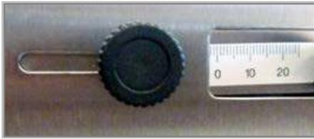
The scale, to the right of the adjusting screw displays the overhang in mm (measured from the outer edge of the sealed seam).
